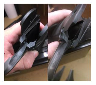
By using a small round edge fine file and working it lightly inside the magazine release channel this will deburr and fit the magazine release to the grip. Because of the large difference in specs on the magazine release, the amount of deburring or fitting will vary between customers.
